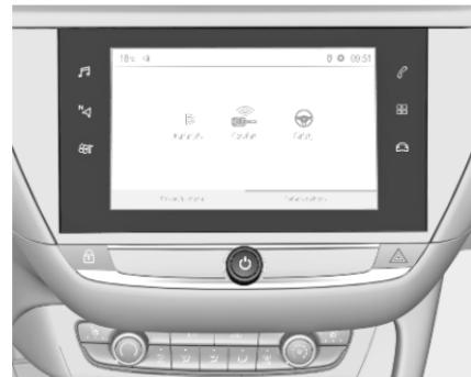
Touch the to open the vehicle personalization menu. Settings for lighting, comfort, and safety can be adjusted.
